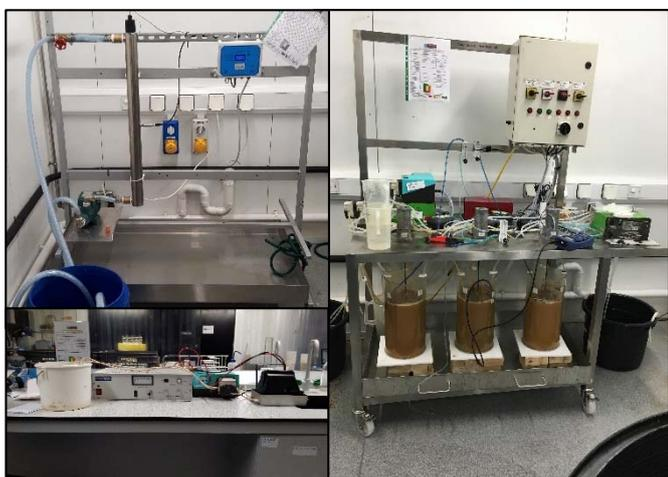
**Laboratory scale experimental equipment at NUI Galway /AIT (Clockwise from top: LPUV, IASBR, PUV)**
